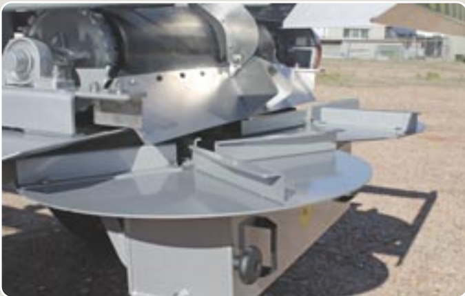
54 Discos, poleas y protector, especial compost Discs, pulleys and protector for special compost machine
