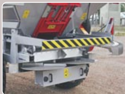
57 Discos, paletas y protector de acero inoxidable hasta 24 m Discs, vanes and stainless steel protector until 24 metres
